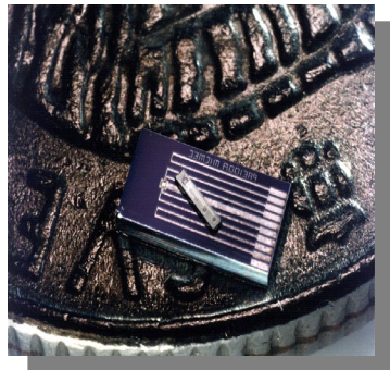
Miniaturised sensor for blood pressure measurements
